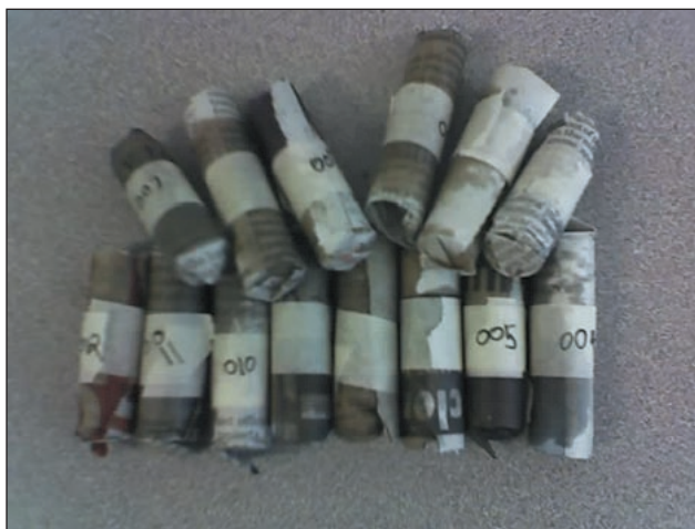
Figure 1. Sample pellets containing biomass (sawdust) and glycerin in a ratio of 1 to 1.3.
